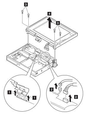
Note: When removing the LCD cables 1, pull the connector straight up. Incorrect handling can damage the connector.
